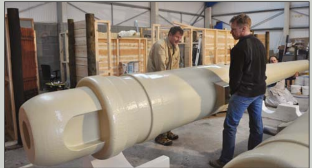
8m long Krupps gun barrels in production
